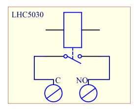
Above schematic outlines how the relay outputs are implemented internally.
