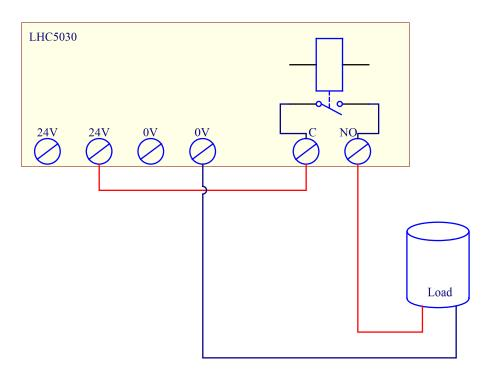
Above schematic outlines an example of how the 24V supply output, together with a relay output, can be used to control a load.
